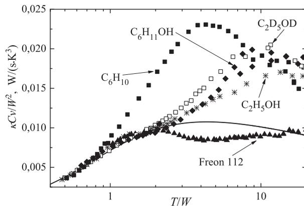
**Fig. 4.** Reduced thermal conductivity  $\kappa(T)\bar{C}v/W^2$  as a function of the reduced temperature  $T/W$ . The symbols mark the experimental data on the thermal conductivity of the orientational glasses of cyclohexanol [4], cyclohexene [18], protonated and deuterated ethanol [2], and freon 112 [3]. The solid line is the universal dependence based on the soft potential model
