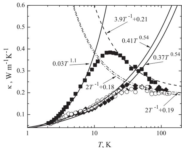
**Fig. 2.** Thermal conductivities of the orientational glasses of cyanocyclohexane (○) [3], cyclohexanol (◆) [4], and cyclohexene (■) [18]. The solid lines show the power law of the thermal conductivity  $\kappa = \alpha \cdot T^n$ . The dashed and dash-dotted lines are the dependence  $\kappa(T) = A/T + C$
