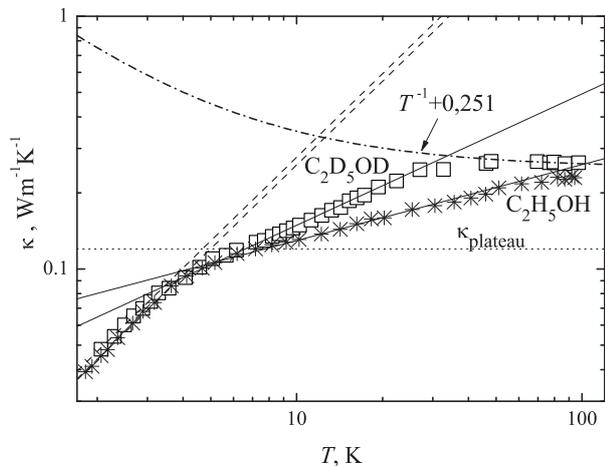
**Fig. 1.** Temperature dependence of the thermal conductivity of orientational glasses of protonated (\*) and deuterated (□) ethanol [2]. The solid and dashed straight lines show the power law of the thermal conductivity  $\kappa = \alpha \cdot T^n$ ; the dotted line is the thermal conductivity at the beginning of the “plateau”  $\kappa_{\text{plateau}}$ ; the dash-dotted line is the dependence  $\kappa(T) = A/T + C$ , where  $A = 1 \text{ Wm}^{-1}$ ,  $C = 0.251 \text{ Wm}^{-1}\text{K}^{-1}$
