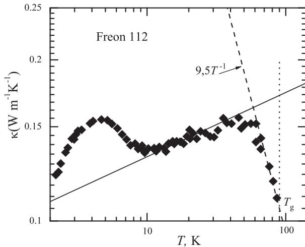
**Fig. 3.** Thermal conductivity of freon 112 in the orientational glass state [3]. The solid straight line is the power law  $\kappa = \alpha \cdot T^n$  describing the behavior of the thermal conductivity. The dotted line shows the glass formation temperature  $T_g = 90$  K
