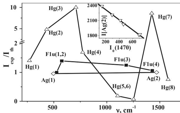
**Fig. 6.** The comparison of observed and calculated intensities of the Raman active  $\text{Hg}(j)$  bands (open symbols) and IR  $\text{F}_{1u}(1-4)$  bands (dark symbols) (*b*). The inset shows the peak intensity decrease for  $\text{Ag}(2)$  band as a function of  $I_0(1470)$  in a vicinity of the current vibration
