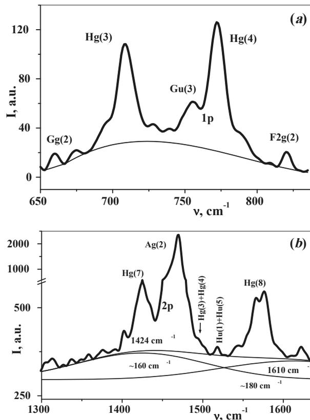
**Fig. 5.** Subtraction of vibrational induced local electronic bands (EB) in the Raman spectra of nanofilms of fullerite  $\text{C}_{60}$  in the case of the hot (*a*) and cold (*b*) methods of deposition and polymerization by diamine in the field of vibrational bands Hg(3,4) (*a*) Ag(2), Hg(7,8) (*b*)
