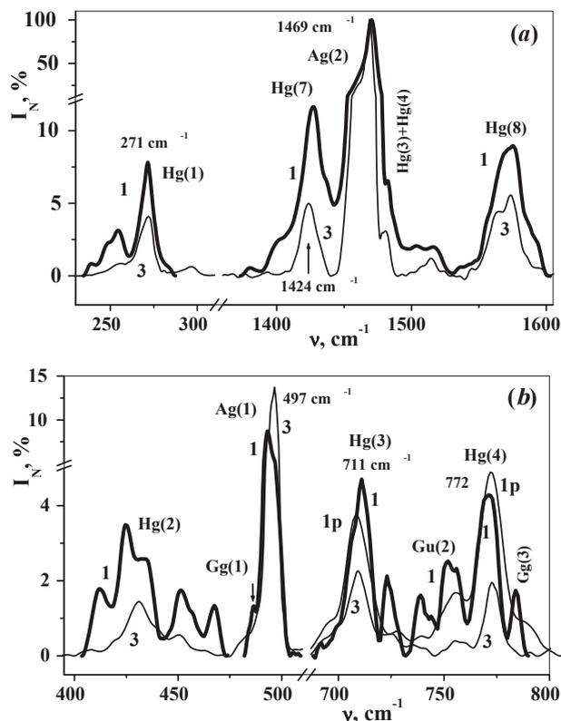
Fig. 2. Comparison of the vibrational bands normalized on line Ag(2) in the Raman spectra of nanofilms of fullerene C<sub>60</sub> fabricated by the hot method of deposition (1), microfilms of fullerene C<sub>60</sub> 2 microns in thickness (3), and nanofilms polymerized by diamine (1p) in the region of the bands Hg(1), Ag(2) and Hg(7,8) and bands Hg(2,3,4) and Ag(1) (*b*)
