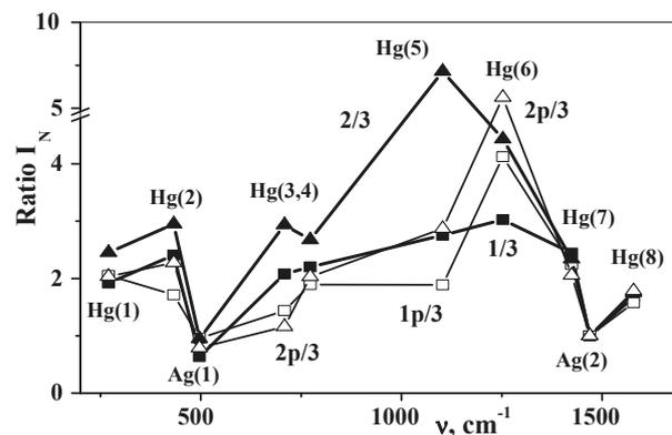
Fig. 3. Enhancement of active vibrations Hg(1–8) in the Raman spectra of the nanofilms of fullerene C<sub>60</sub> in comparison with microfilms about 2 microns in thickness in the cases of the hot (1/3) and cold (2/3) deposition methods, as well as nanofilms polymerized by diamine (1/3 and 2p/3)
