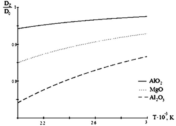
**Fig. 3.** Dependence of the relative diffusion coefficient  $\frac{D_z}{D_0}$  on the temperature for various molecules of oxides
