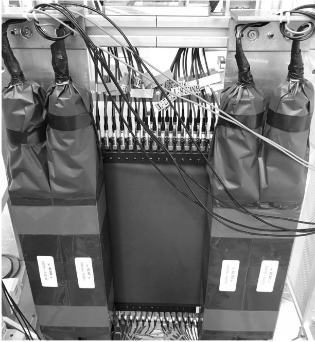
Fig. 8. Beam Monitor: The LEMO readout connectors of two offset planes are seen, continued with bigger BC-404 scintillators. The beam hits into the picture
