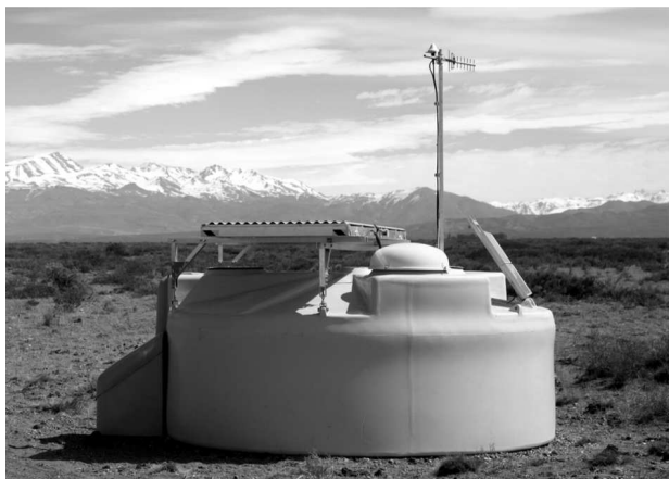
Fig. 7. Photograph of an upgraded station of the SD, featuring the SSD on top of the WCD
