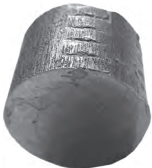
Fig. 9. A deformation well (hole) on the surface of a continuously cast Бр08Н4Ц2-bronze billet at 100 °C
