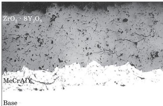
Fig. 8. The microstructure of barrier coating. Reproduced with permission from M. Hetmanczyk *et al.*, *J. of Ach. Mater. Manuf. Engin.*, **24**, No.1: 372 (2007); [https://www.researchgate.net/publication/40804836\\_Advanced\\_materials\\_and\\_protective\\_coatings\\_in\\_aero-engines\\_application](https://www.researchgate.net/publication/40804836_Advanced_materials_and_protective_coatings_in_aero-engines_application). Copyright 2007, International OCSCO World Press [101]
