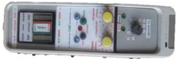
Fig. 4 Two-channel programmed myostimulator "MyoBalanceStimul"
