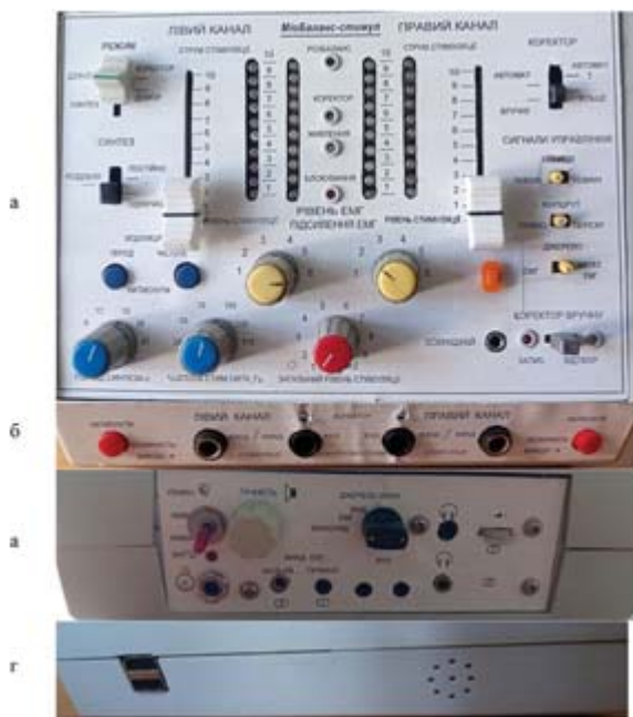
Fig. 7. Two-channel programmed myostimulator "MyoBalanceStimul-2". Device layout
