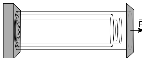
Fig. 1. Deformation of MWCNT with shells of unequal lengths. Imposed force is applied only to the external shell
