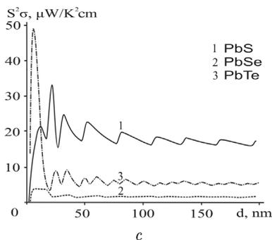
**Fig. 3.** Theoretical dependences of the Seebeck coefficient  $S$  (a), electric conductivity  $\sigma$  (b), and TE power factor  $S^2\sigma$  (c) on the QW width for films of PbS (1), PbSe (2), PbTe (3) in the model of infinitely deep potential well at  $T = 300$  K
