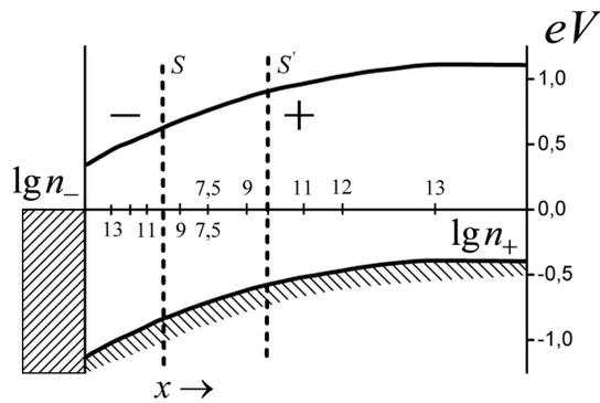
**Fig. 8.** The very first diagram of a  $p$ - $n$  junction (taken from work [12]). The region of  $p$ -conductivity is located to the right from the vertical line  $S'$ , and the region of  $n$ -conductivity to the left from the vertical line  $S$ . The numbers below and above the abscissa axis indicate the logarithms of the hole ( $n_+$ ) and electron ( $n_-$ ) concentrations
