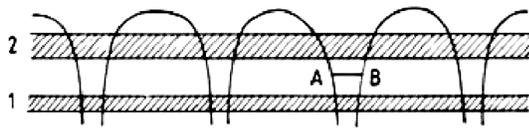
Fig. 5. The very first band diagram of a semiconductor from Wilson's work
