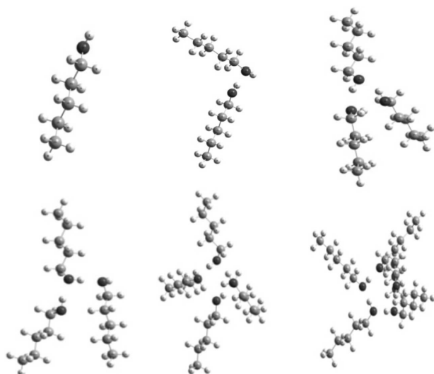
Fig. 2. Optimized structures of different clusters of n-pentanol
