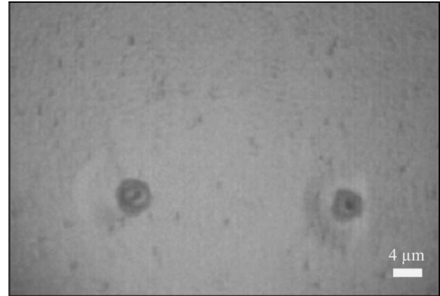
Fig. 4. Optical microphotos of the surface of a tested specimen. Two concentric spots are typical traces of the action of a 10-mW laser beam
