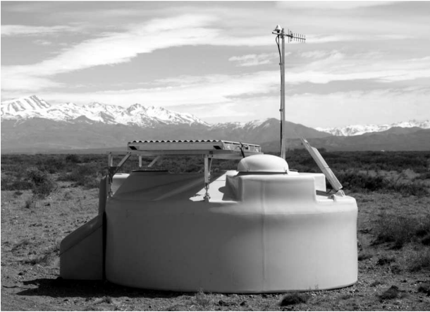
Fig. 7. Photograph of an upgraded station of the SD, featuring the SSD on top of the WCD
