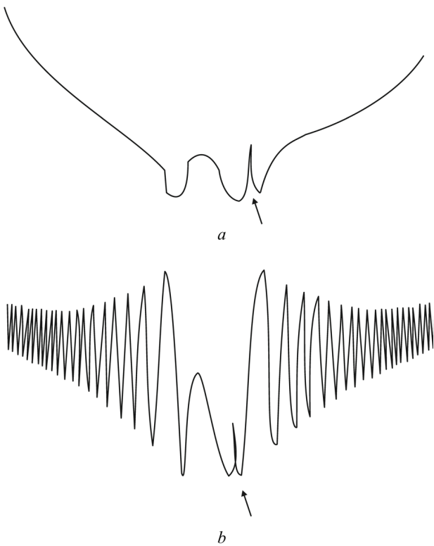
Fig. 6. Dependences of the weaker-wave intensity change (a) and the beat frequency of counter-propagating waves (b) on the laser generation frequency
