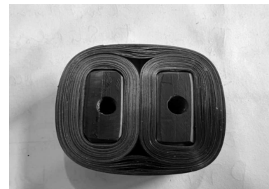
Fig. 3. Amorphous core shapes and sizes
