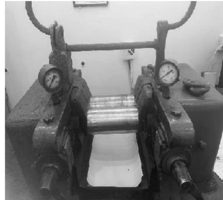
Fig. 2. Rolling device EZM 50 for the deformation of amorphous ribbons by rolling
