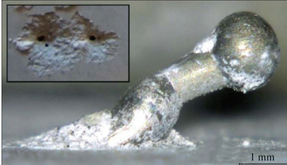
Fig. 16. Die cutting failure of concrete-pin connection
