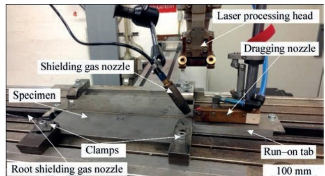
Fig. 2. Experimental setup for the laser welds
