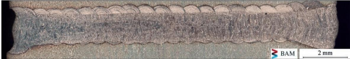
Fig. 4. Microsection of weld seam with LMD-tacking
