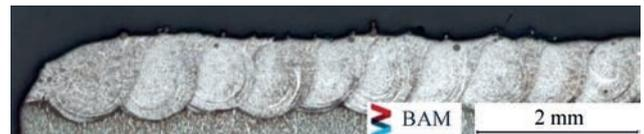
Fig. 3. Cross section of buttering of edges
