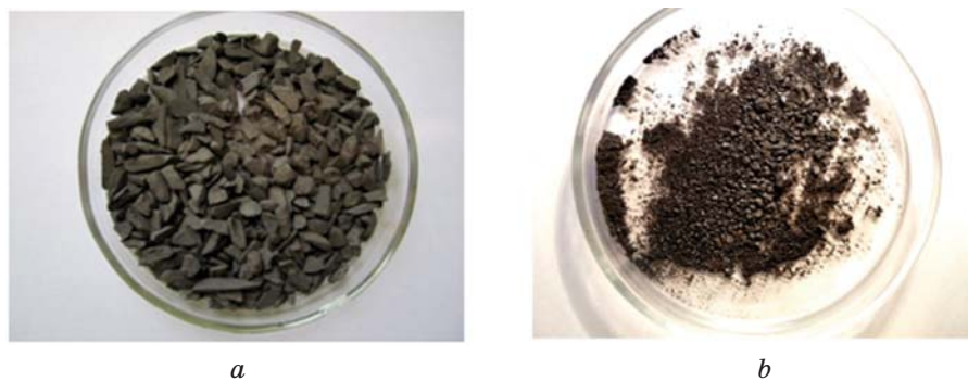
Fig. 5. Appearance of black waste dumps: before (a) and after (b) bacterial leaching with nutrient medium A-27
