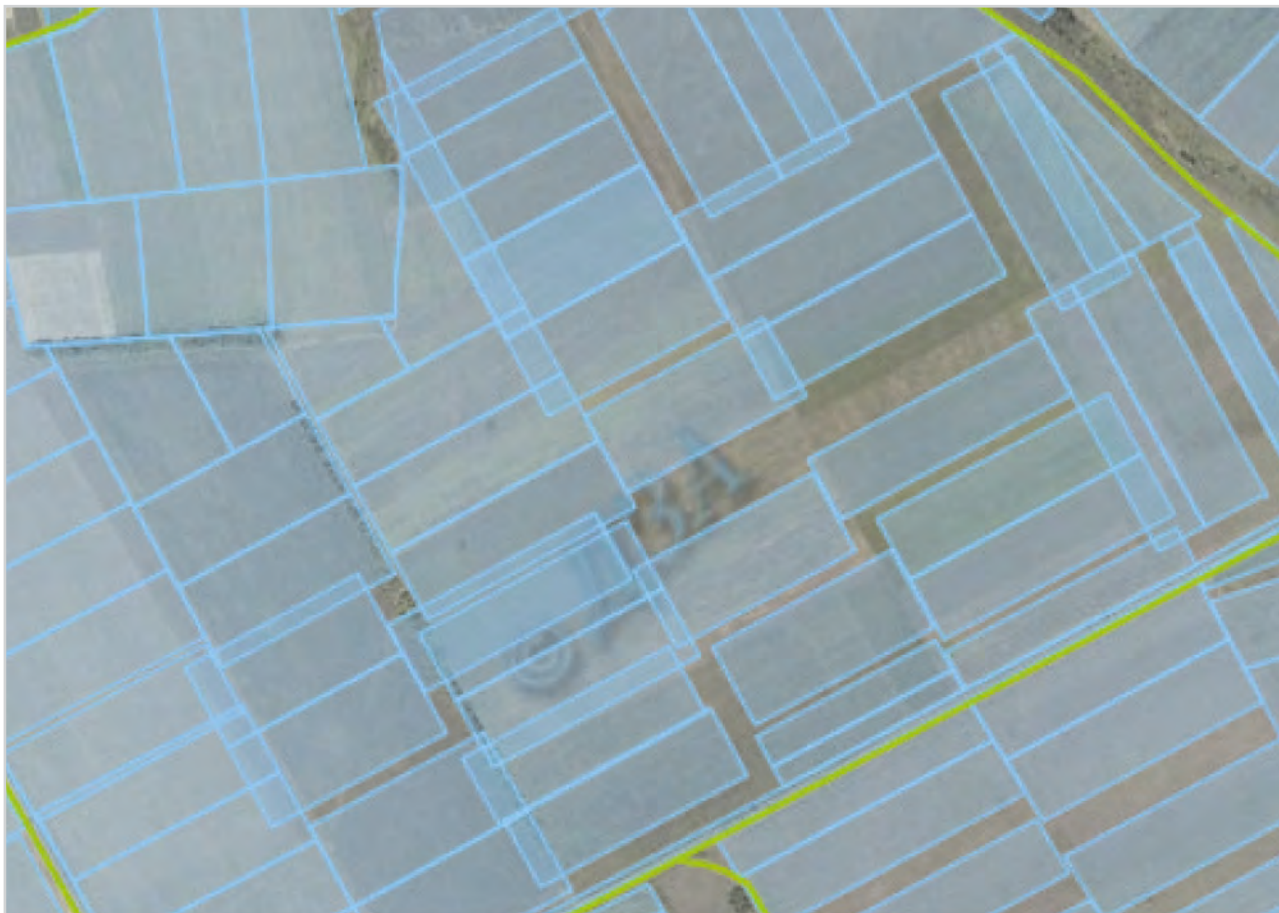
Figure 1: Example of technical errors in the database of State Land Cadastre Source: Public cadastral map of Ukraine
