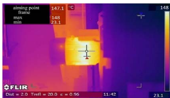
Fig. 3. A thermogram of the induction generator
