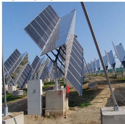
Fig. 1. Example of SGM module, equipped with a one-sided low solar concentration system
