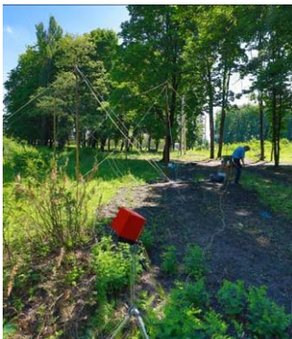
Fig. 12. Picture of magnetic field sensor spatial arrangement outside the shielding space for open loop control by system of active shielding model
