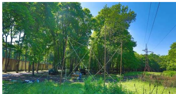
Fig. 2. Picture of the both shielding coil, the spatial arrangement of which were chosen without system synthesis
