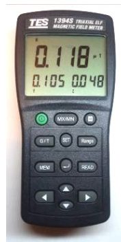
Fig. 9. Three-coordinate magnetometer for measuring resulting magnetic field
