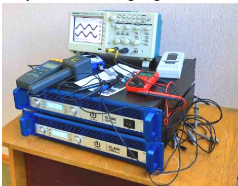
Fig. 7. Power amplifiers for powering compensation windings
