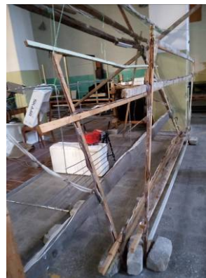
Fig. 12. Two compensating windings of active shielding system
