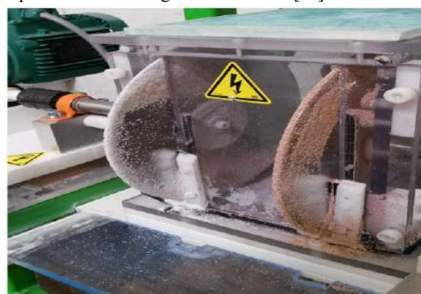
Fig. 2. Collection of insulating particles in the two-rotating-disk tribo-aero-electrostatic separator
