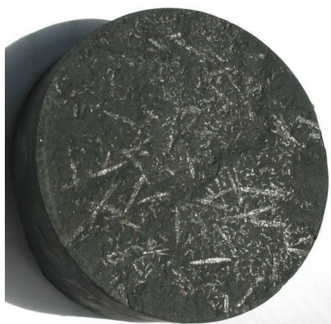
Fig. 2. Shows the typical appearance of Silurian black massive graptolitic argillites enriched with organic matter in core for the section of the parametric well 1-Lishchynska: sample Lishch. 1-66, depth interval 3450–3454 m, core – 78 mm
