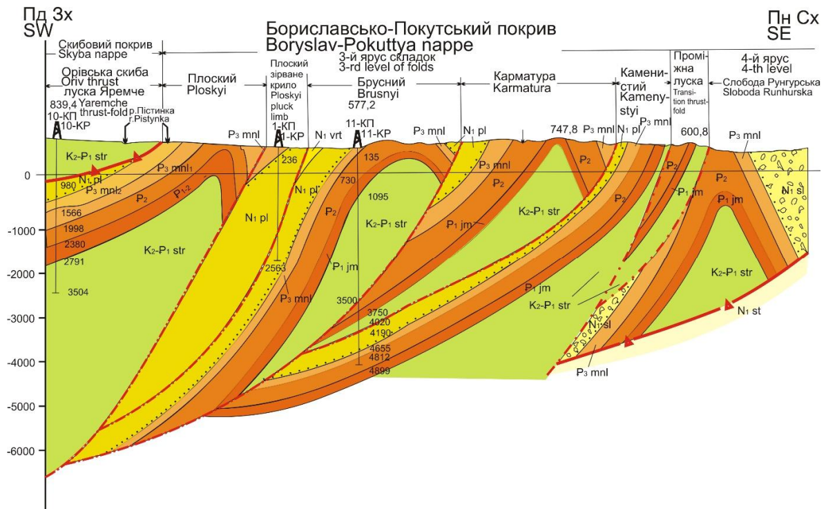
Fig. 4. Geological cross-section along the line of boreholes 10-11-Kosmach-Pokutskyi (Legend see Fig. 2)
