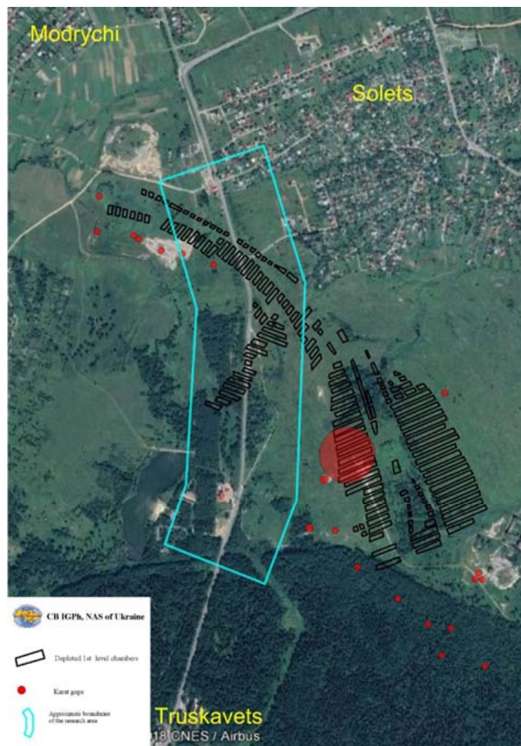
Fig. 1. Area of electrical prospecting in the limits of mining field No. 2 of Stebnyk potassium deposit
