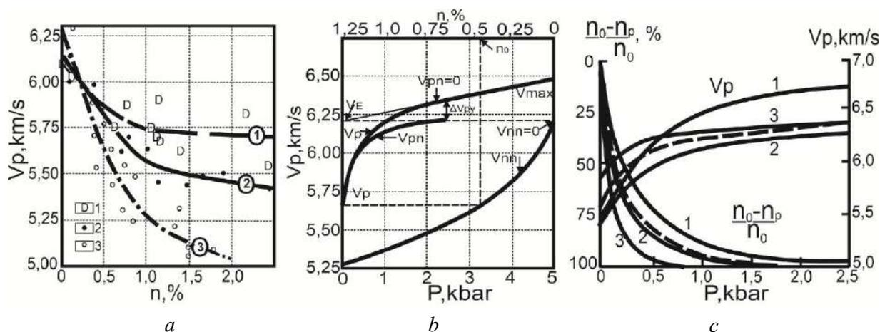
**Fig. 3.** Changes in velocity and pore space with pressure in granites:
