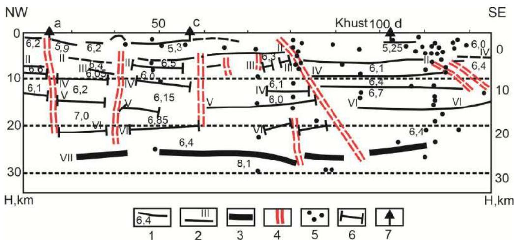
**Fig. 7.** Seismic section of the Earth's crust and local earthquake hypocentres along the TD [Chekunov et al., 1969; Tretyak et al., 2015; Nazarevich, Nazarevich, 2004; Nazarevich et al, 2002, 2011]. 1 – refraction layers and velocities along them; 2 – reflection horizons and their numbers; 3 – Moho discontinuity; 4 – faults; 5 – earthquake focuses; 6 – seismic boundaries; 7 – hydrocarbon exploitation wells
