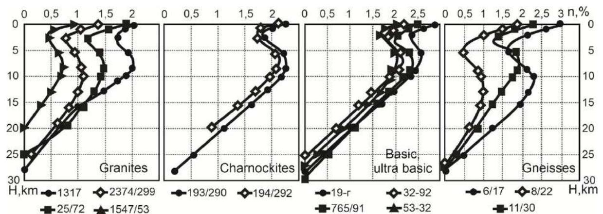
Fig. 4. Change in porosity of the crystalline rocks under thermodynamic conditions at the different depths
