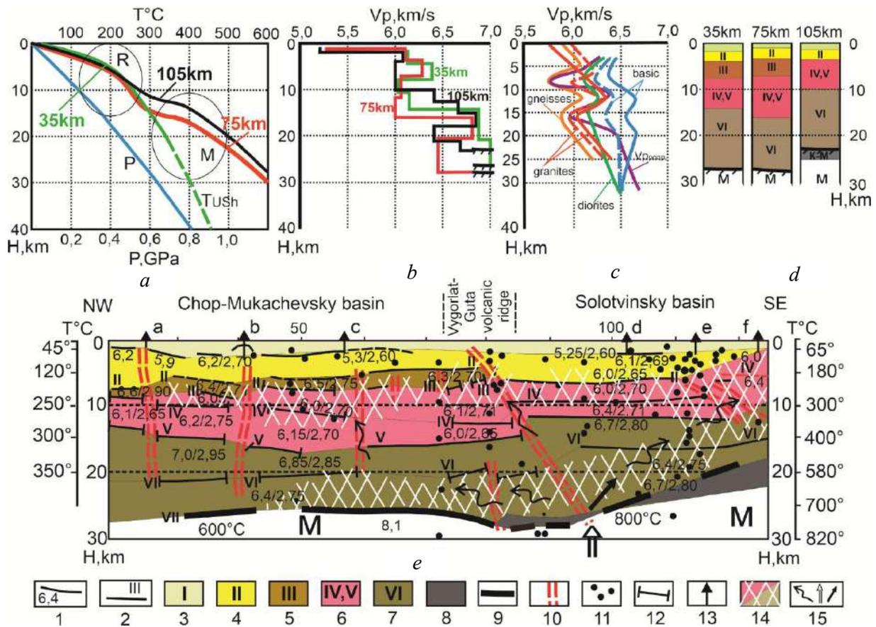
**Fig. 8.** Elements of PTBM for areas of 35, 75, 105 km of the RP-17 DSS profile (a–d) and the model of rocks distribution with a depth along TD (e) (this study and data from Chekunov et al., 1969; Tretyak et al., 2015; Nazarevich, Nazarevich, 2004; Nazarevich et al, 2002, 2011):
