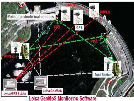
**Fig. 3.** Scheme of the stationary system for monitoring the spatial displacements of the Dnipro HPP buildings.
