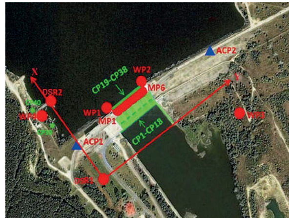
Fig. 4. Geodetic SSMSDS network of the Dnister HPP-1
