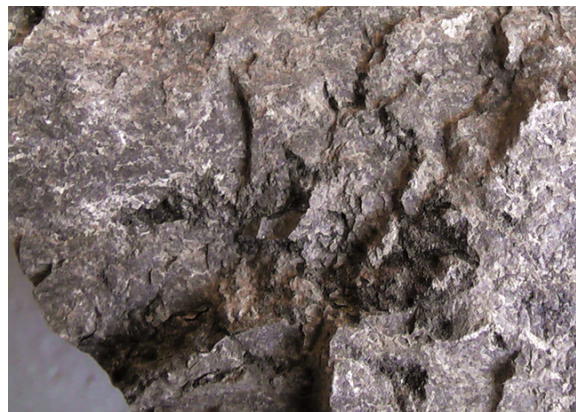
Fig. 1. Adiabatic fractures of limestones from borehole 1 Machukhy, interval 5197–5214 m, the yield of core is 25 %.
