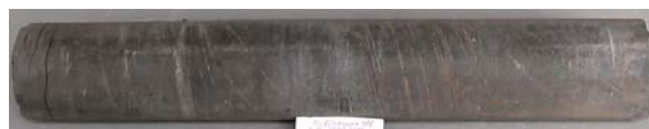
Fig. 3. Dense limestones from borehole 479 Novodykanka, interval 4565–4580 m, the yield of core is 89 %.
