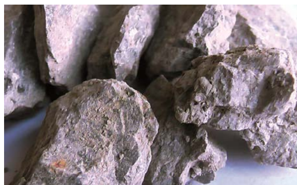
Fig. 2. Adiabatic fractures of limestones from borehole 2 Machukhy, interval 5247–5262 m, the yield of core is 17 %.
