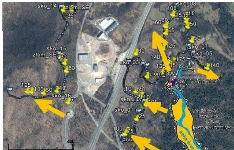
Fig. 16. Georadar profiles above and westerly of Škocjan Caves
