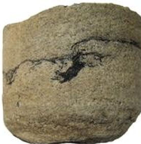
Fig. 5. Photo of the core with cavities and cracks from well 17-Semyrenkivska.
