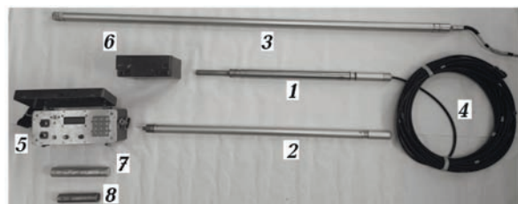
Fig. 2. Prototypes of new radioactive logging tools and support equipment: 1 — 2NNL tool, 2 — DL+GR tool, 3 — TRL tool, 4 — logging cable, 5 — surface console, 6 — accumulator, 7 — chamber of \gamma -ray source, 8 — chamber of neutron source.
