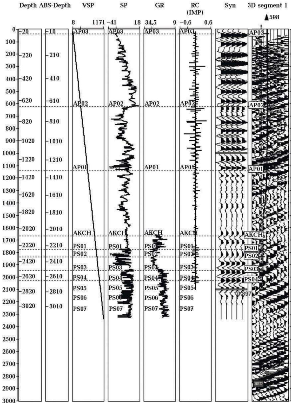
Fig. 7. Seismo-acoustic model for a section of Well598.
