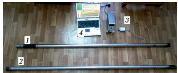
Fig. 2. Pilot sample of the universal UMRL module: 1 — submodule 2GGL+GR, 2 — submodule 2NNL+2NGL, 3 — power supply unit, 4 — software unit.
