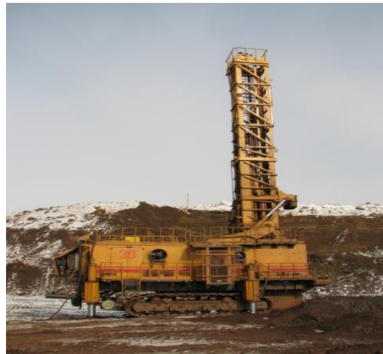
Figure 5 - Drilling machine CBIII- 250MHA-32KII with compressor unit BB-50/8Y2
