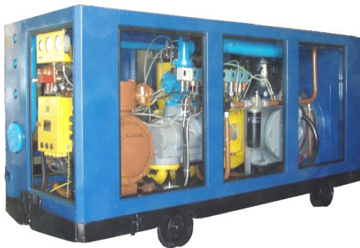
Figure 3 – The shaft screw compressor unit УКГШ-10/7 A Y2 with electric protection system
