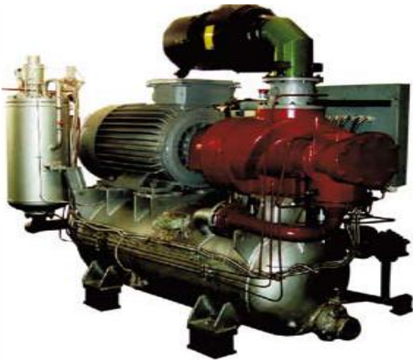
Figure 4 – The compressor unit for drilling machine
