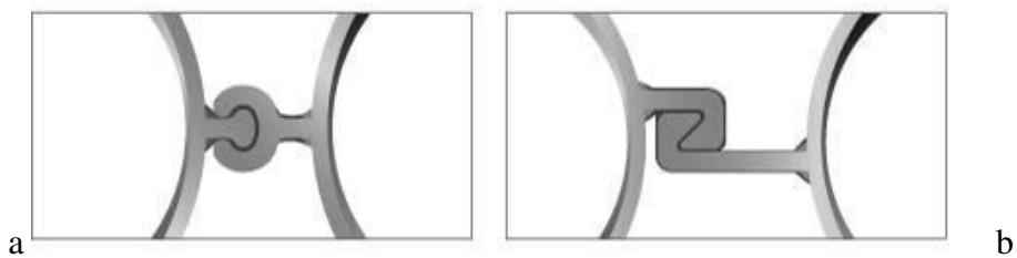
Figure 15 - Types of lock elements of pile wall technology; a - lock type WoM/WoF; b - lock type C6
