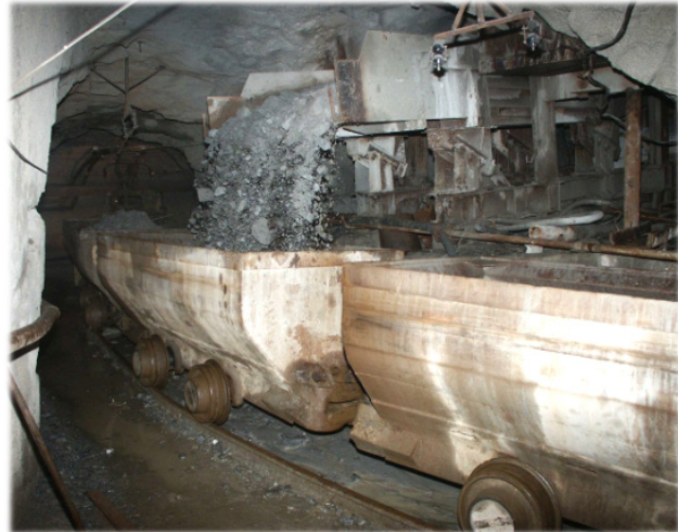
Figure 2 – Vibratory feeder of the VPR-4m type for the ore drawing and feeding from the panel to the wagons
