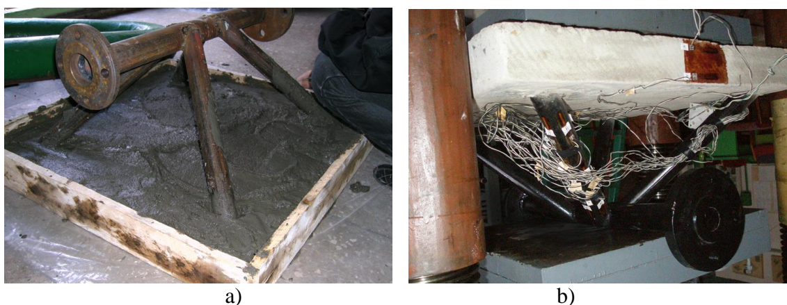
Figure 4 – It is the combined structural elements while production (a) and testing under uniform load (b)
