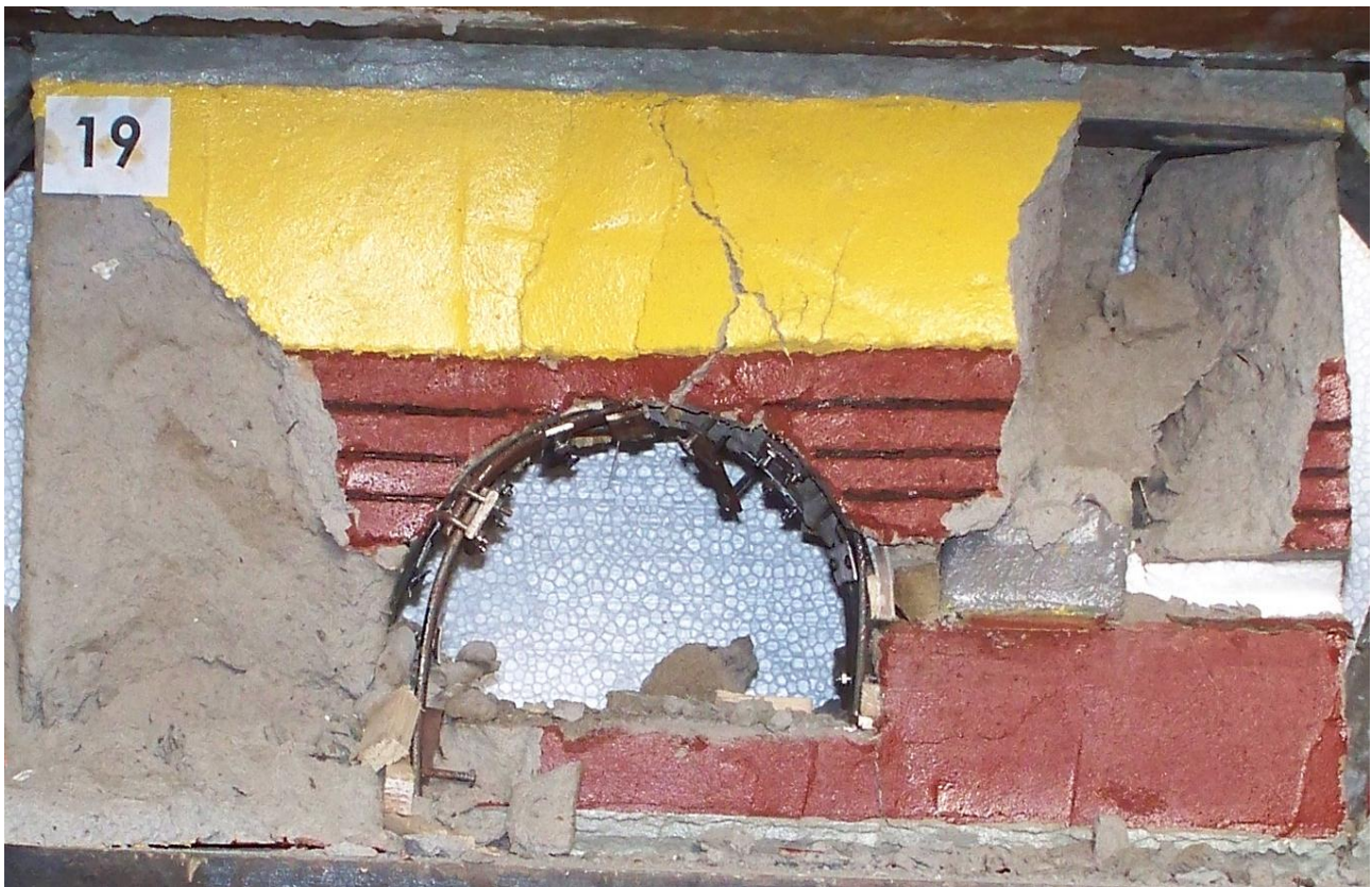
Figure 9 – Racks pressed into the floor of a working for model #19
