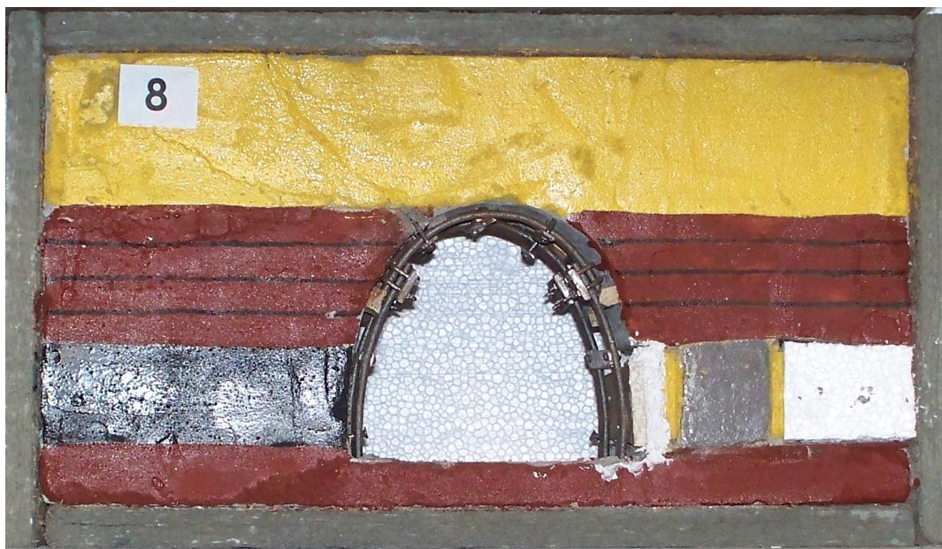
Figure 5 – Model #8 set up prior to experimental study
