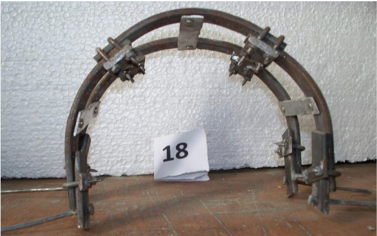
Figure 8 – The shape of the five-element frame after the test completion
