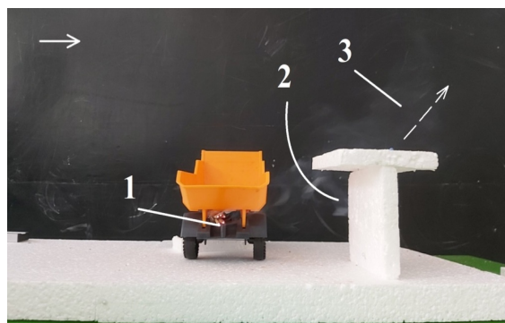
1 – place of emission of pollutant; 2 – area of contamination under the plate; 3 – area of contamination above the plate
