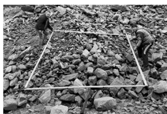
Figure 3 – Measurement of granulometric composition of the blasted rock mass on the ledge of the granite open pit
