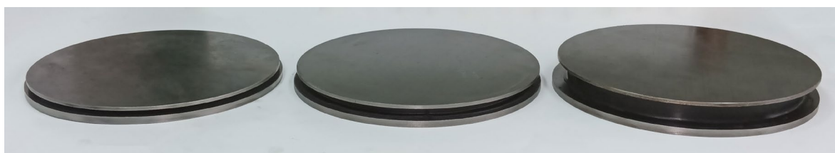
Figure 2 – Different sizes of vibration isolators that were subjected to laboratory tests
