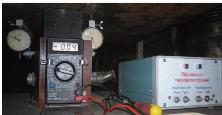
Figure 2 – Appearance of an inertia-free stress and strain recorder for testing rock specimens
