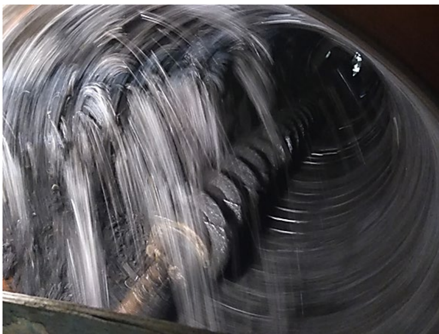
Figure 5 – Waterfall mode of the wet material movement inside the screen drum rotating with a frequency of 40 rpm
