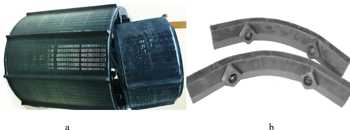
Figure 4 – Sieving component forming DABS (a) and rubber lining elements of places where DABS parts are fixed to the screen drum (b)
