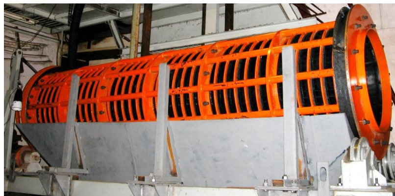
Figure 1 – Full-size drum-like screen with a working surface DABS within the test bench of the research
