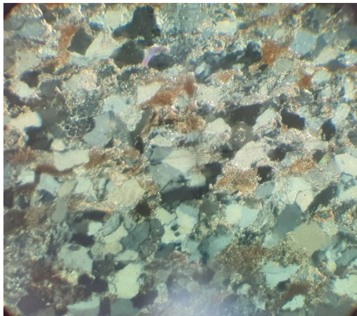
Figure 2 – Outburst-hazardous sandstone d_3Sd_4 from the Pokrovsk mine, coastal marine facies, fine-grained, sorted, weakly rounded, little altered, thin section, magnification 100^X
