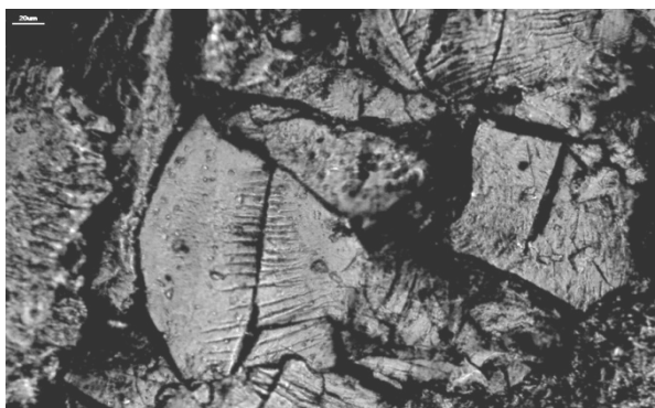
Figure 4 – Brittle and plastic deformation in a single coal particle
